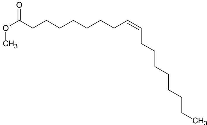
Although structurally rather different to conventional diesel, FAME can be successfully blended with conventional diesel at a variety of dose rates, or used as a pure road fuel in modified engines.
