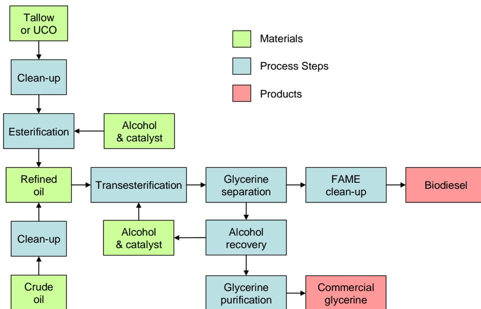
Triglycerides from vegetable oil or animal fats are converted by transesterification with a base catalyst and methanol to fatty acid methyl esters (FAME) and glycerine. The methanol replaces the glycerol which is released for recovery. The FAME is purified for use as biodiesel and the glycerine purified for sale into other markets as a co-product.
