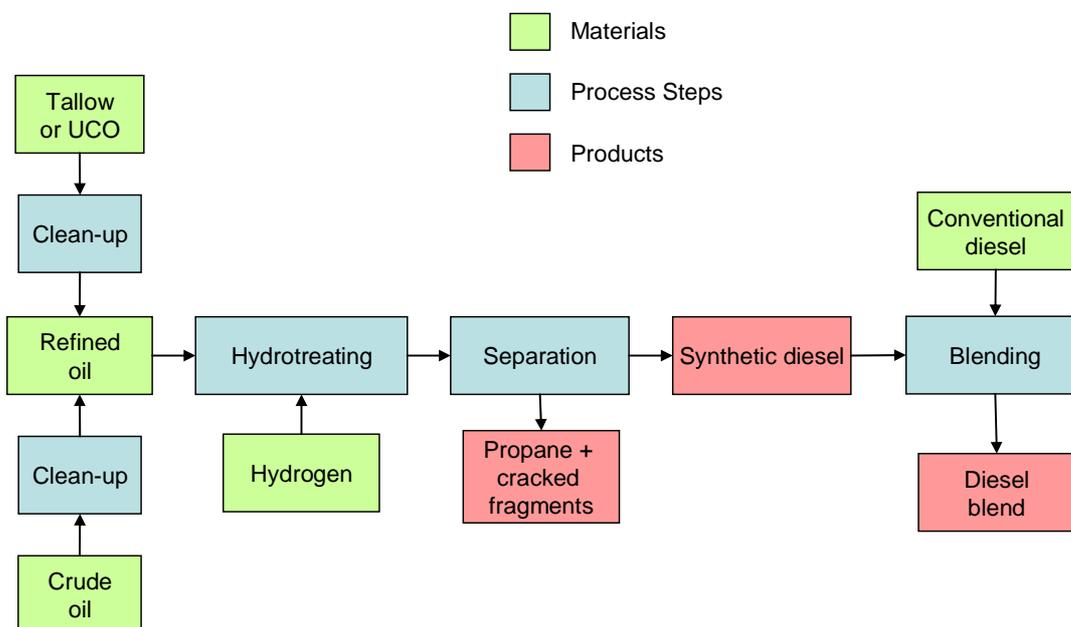
The oils and fats are treated with hydrogen in the presence of a catalyst. This breaks the glycerol from the fatty acids, removes all oxygen and removes any double bonds. The glycerol is converted to propane, and together with any fragments created by the hydrogenation process is separated and used within the refinery. The synthetic diesel is a very high quality product that is chemically identical to conventional diesel.
